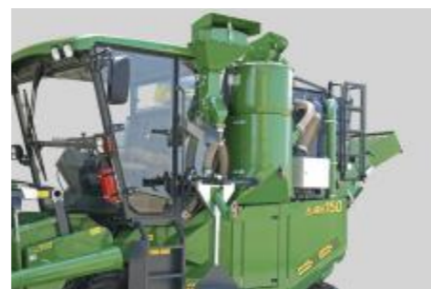
Different weighing systems offer customized solutions: plot weight, moisture analysing, test weight, and NIRS. Harvest Master available.
