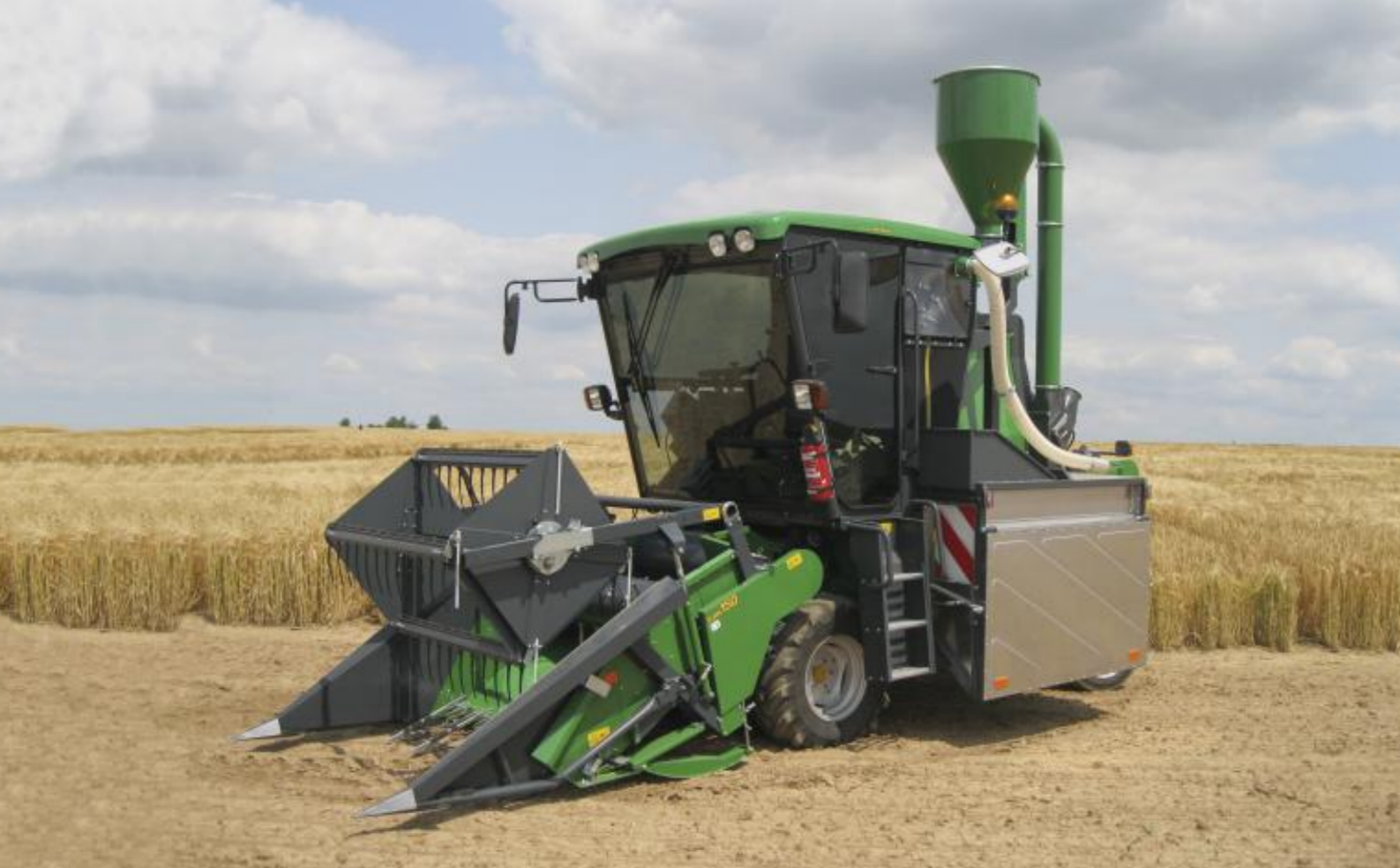
Grain Header with conveyor belt, intake auger and feeding roller for a perfect flow into the threshing system.
