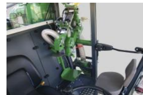
The bagging and sampling system offers various functions and dust-free bagging in- and outside the cab.
