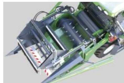
Grain Header with conveyor belt, intake auger and feeding roller for a perfect flow into the threshing system.
