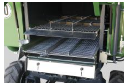
3 step surface shaker and double-sieve system: better cleaning results due to top and bottom sieve.
